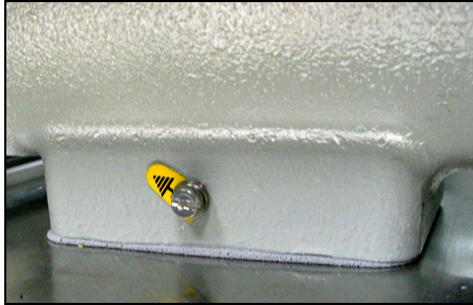
Figure 30: Earth Ground Connection
