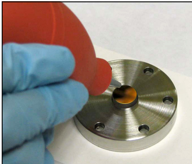
Figure 82: Blowing Air onto the Mirror
