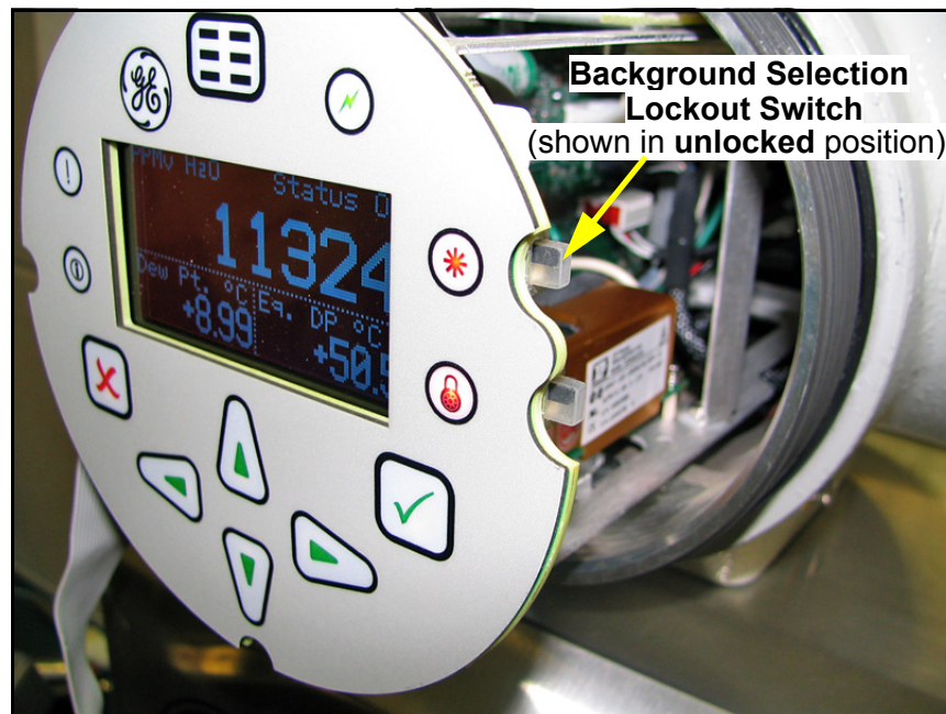
Figure 101: Background Selection Lockout Switch Location
