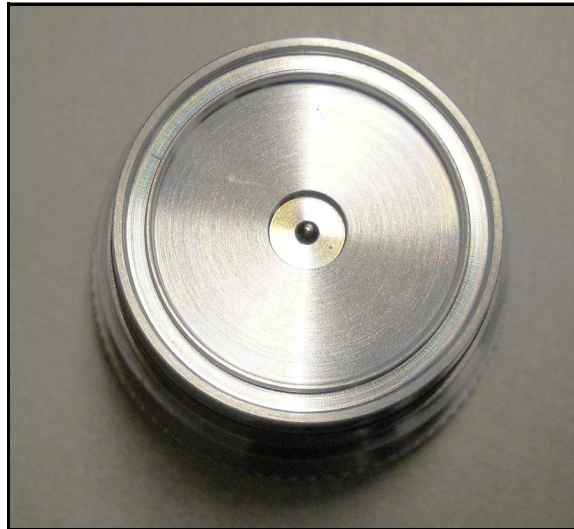
Figure 97: Remove the Small O-ring
