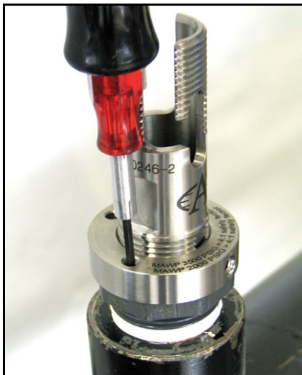
Figure 15: Tightening the Allen Screws
