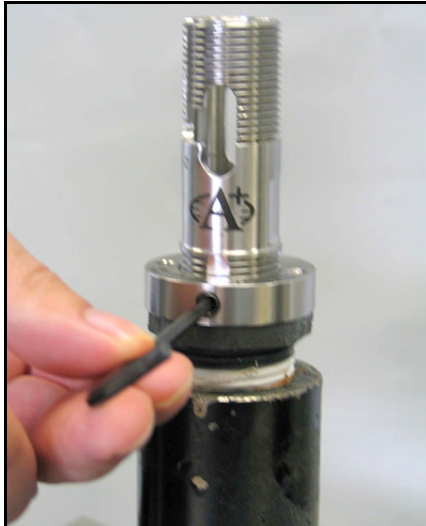
Figure 14: Aligning and Tightening the Allen Screw
