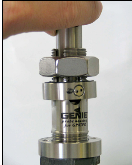
Figure 20: Rotating the Probe
