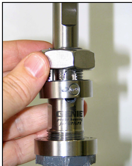
Figure 21: Loosening the Insertion Nut
