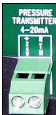
Figure 29: Pressure Transmitter Connections
