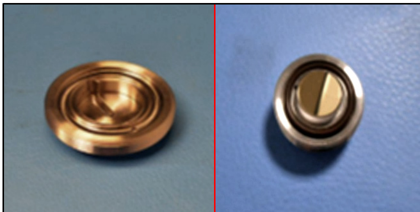
Figure 91: Replacing Cleaned Mirror into End Cap Assembly
