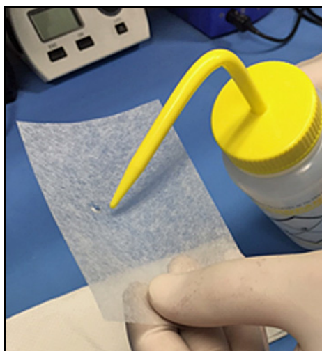
Figure 89: Applying Acetone to Lens Tissue
