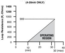
Loop Supply Voltage (Vdc) [LSV]
