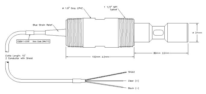
ES-5-A 4-20 mA output, CPVC body with 1.5" MNPT thread fitting
