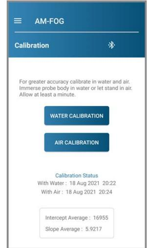
Note that the Calibration screen reports the results of the calibration: the date of both calibrations and the slope and the intercept of the graph that converts frequency values to the calibrated range of 0 to 10,000.
