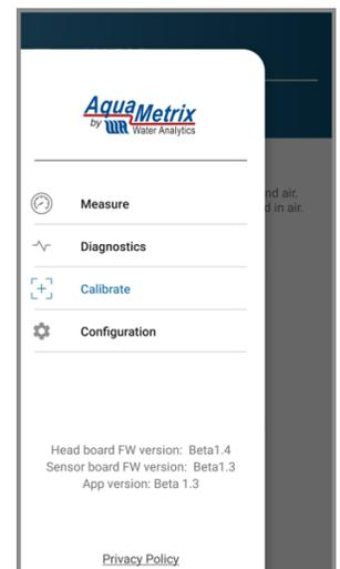
To calibrate the probe, press the menu icon in the top left and bring up the menu screen (right). Select **Calibrate**.
