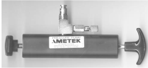
If you want to check/calibrate manometers, transducers or transmitters, it is a good idea to use a hand pump to generate pressure for the test. This pump can be delivered with all EPM systems, but may also be purchased separately.
