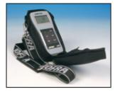
the pressure module connector. A shoulder strap ensures convenient transportation when climbing ladders, etc. and the handy strap at the back makes it possible to hang the instrument on a pipe, ladder etc, while performing the calibration, test, or service task.
