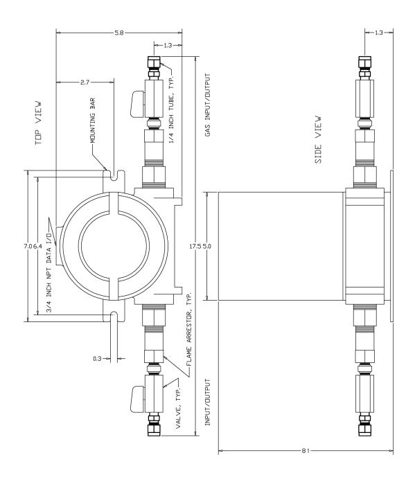
Figure 3.0 Series 3500 with NEMA 7 Enclosure
