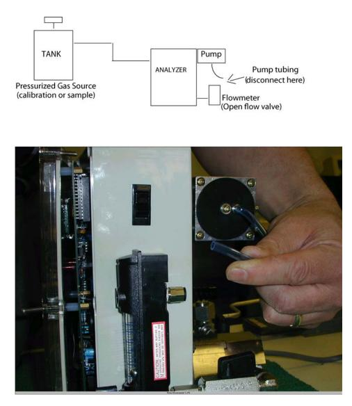
Disconnect tubing at the flow meter
