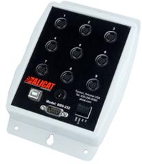
The Multi-Drop Box has nine 8 pin Mini-DIN ports available. The ports are to be used with a standard double ended 8 pin Mini-DIN (DC-62) style cable going from the box to each flow or pressure device. (The BB9 can also be ordered with locking industrial connectors.)
