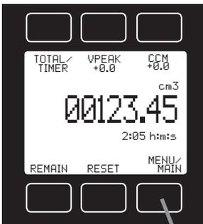
If your meter was ordered with the **Totalizer** option (page 45), pushing the **TOTAL/MENU** button once will bring up the **Totalizing Mode** display. Pushing **MENU** will bring up the **Select Menu** display.
