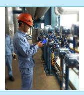
The demands of remote calibration work can be challenging. The ADT227series is lightweight and highly portable and utilizes an advanced color LCD screen to help ensure you can easily see, even in the (Ex) intrinsically safe versions.
