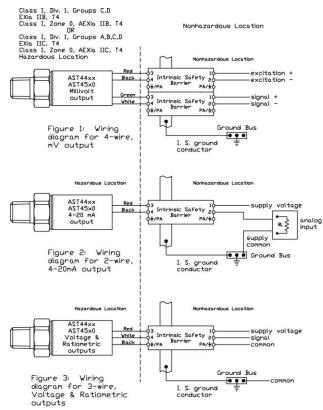
Models AST4400, AST44LP, AST4500, AST4510, AST4520, AST4530 Class I, Div. 1, Groups C,Dj EXia IIB, T4; Class I, Zone 0, AEXia IIB, T4 vax=28Vdc
