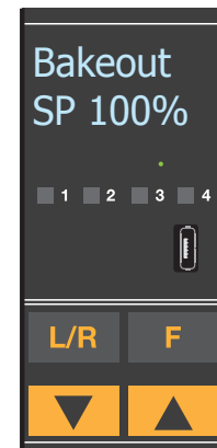
Heater Bakeout Indication
