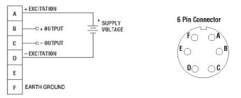
**NOTE:** Completion of the earth ground (Pin F) is recommended for proper circuit protection.
