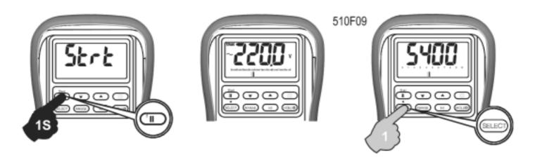
Press the **Start** button momentarily to pause or to continue. The LCD annunciator "H" will be flashing when paused.
