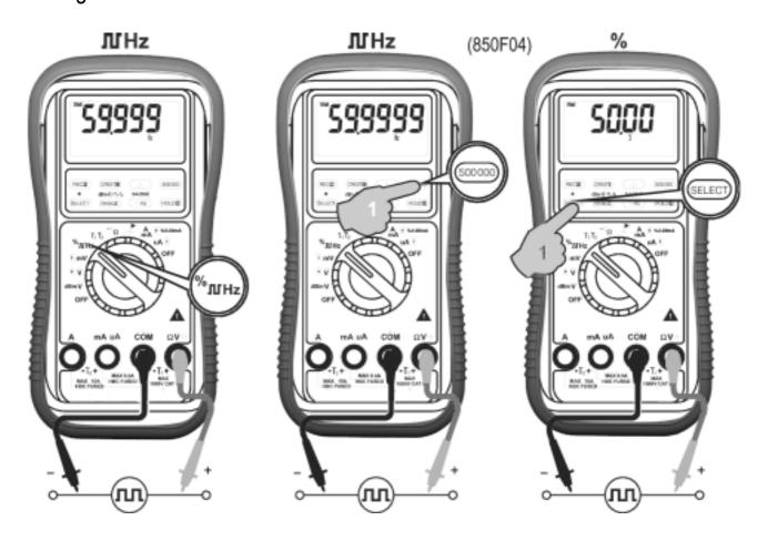
Note: Unlike the Line Level Frequency measuring function as previously stated, this Logic Level Frequency function is set only at the highest input sensitivity to measure digital type electronic signals.
