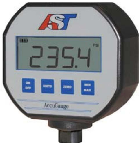
The AG100 series is a 9V digital pressure gauge featuring multiple measurement units, min/max readings, selectable tare/zero and an automatic power off to conserve battery power. Also, a backlight provides improved visibility under marginal lighting conditions.
