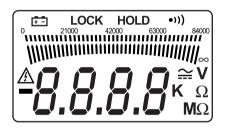
LOCK High Voltage Output Lock Enable
