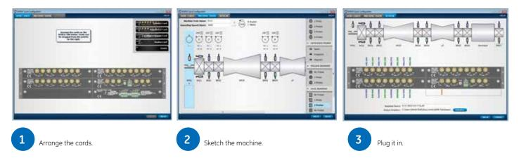
The ADRE Quick Configuration Software allows even the novice user to create an Sxp-ready database to configure ADRE and start receiving data within minutes. Bently best practices are integrated into the wizard to automatically create data collection parameters and a suite of plots to ensure the full power and productivity of the ADRE system is realized.
