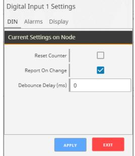
There is a Digital Input tile for each of the two digital inputs, unless they are configured for Flow Mode. If the 2AI/1DI expansion card is installed, it will appear as its own Digital Input 3 tile.
