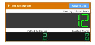
If the Ranger is configured with the SDI-12 expansion card, the SDI-12 tile will appear on its Cloud page. Click on "Configure" to set up the values for the Ranger to read. To add a line, click on the "+" button, and specify the value name, sensor address, SDI-12 request, and which position of the response to read in. To remove a line, click on the trash can icon followed by clicking "Delete Rows". Hit Apply to set the lines, and the Ranger will begin reading the values specified in the table.
