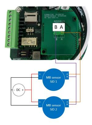
Sensor powered by external source
