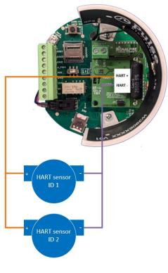
Sensor powered by Ranger. Jumper is on.
