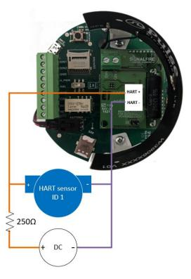
Sensor powered by external source. Jumper is off.
