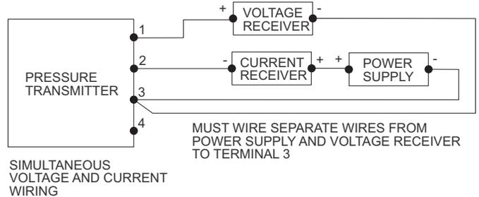
For the current output, the maximum allowable loop resistance (wiring + receiver resistance) is dependent on the power supply. The maximum loop voltage drop must not reduce the transmitter voltage below 17 V. The maximum loop resistance can be calculated using the following equation:
