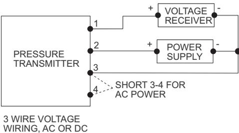
The minimum receiver load is 1K  $\Omega$ . The resistance due to the wire should be low compared to the receiver load resistance. While the voltage at the terminal block remains unchanged with a 10 mA current flow, resistive losses in the wiring do cause errors in the voltage delivered to the receiver. For a 1% accurate gauge, the resistance of the wires should be less than 0.1% of the value of the receiver load resistance. This will keep the error caused by the current flow below 0.1%.
