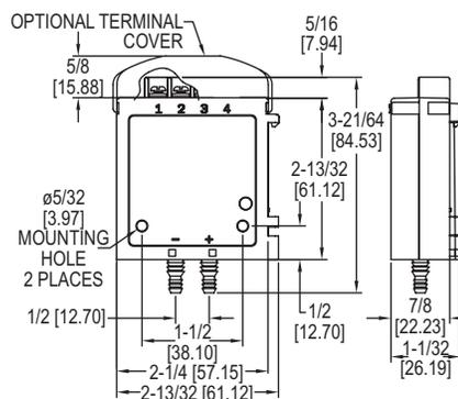
The **SERIES 616KD-LR** Low Range Differential Pressure Transmitter senses the pressure of air and compatible gases and sends a standard 4 to 20 mA and simultaneous voltage output signal. A wide range of models are available factory calibrated to specific ranges including low ranges down to 0.1 in w.c. (25 Pa). New enclosure enables the 616KD-LR to be mounted on a 35 mm DIN rail either via its side or back DIN rail clips. The 1/8" NPT process connection is also available in the Series 616KD-LR.
