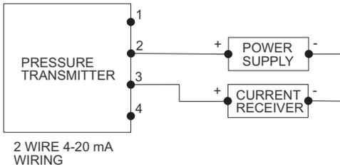
The range of appropriate receiver load resistances ( $R_L$ ) for the power supply voltage available is given by the formula listed below. Shielded 2-wire cable is recommended for control loop wiring. Ground the shield at the power supply end only.
