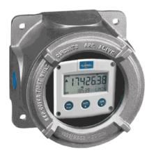
CSA approved explosion proof for hazardous environments, the loop powered level indicator displays engineering units connected in series with one 4-20 mA continuous level transmitter. Select this level indicator for hazardous applications with an explosion proof level sensor. The windowed field enclosure is wall mounted.
