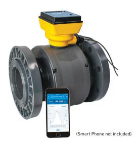
The Signet 2580 FlowtraMag is a full-bore plastic in-line style magnetic flow meter. The PVC body with titanium electrodes has no moving parts, and is two to three times lighter in weight compared to traditional metal magmeters on the market. It is designed for high accuracy flow measurement in short pipe runs, making it an ideal solution for industrial applications where performance and simplicity are important.
