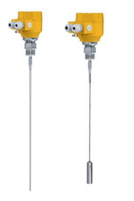
The 2291 Guided Wave Radar level transmitter is designed for continuous level measuring of conductive or non-conductive liquids, pulps and solids. The 2291 level gauge operates based on the well-known TDR (Time Domain Reflectometry) principle. Micropulses are sent along a probe guide at the speed of light. As soon as the impulse reaches the surface of the medium, it is reflected back to the electronic module. Level distance is directly proportional to the flight time of the impulse.
