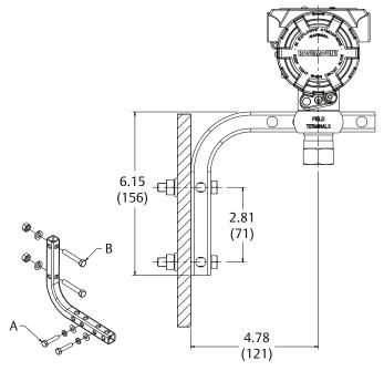
A.  $^1/4 \times 1^1/4$  bolts for transmitter mounting B.  $^5/16 \times 1^1/2$  bolts for panel mounting (not supplied) Dimensions are in inches (millimeters).
