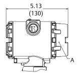
A. Digital display cover B. 2<sup>1</sup>/2–14 NPT conduit connection Dimensions are in inches (millimeters).
