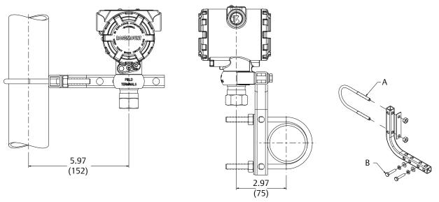
A. 2-in. U-bolt for pipe mounting (clamp shown) B.  $^1/4 \times 1^1/4$  bolts for transmitter mounting Dimensions are in inches (millimeters).
