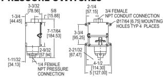
With extremely rugged construction the **SERIES 1000W** provides excellent reliability in chemical, petroleum and industrial plants. Bellville spring movement permits mounting of control in any position and helps prevent contact chatter. New design also provides high over-pressure protection. Weatherproof housing is standard.
