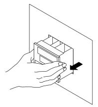
5. The location and number of the relays differ depending on the model code of the UT550/ UT520 Confirm the location of the control output relay to be replaced before pulling out the relay.
