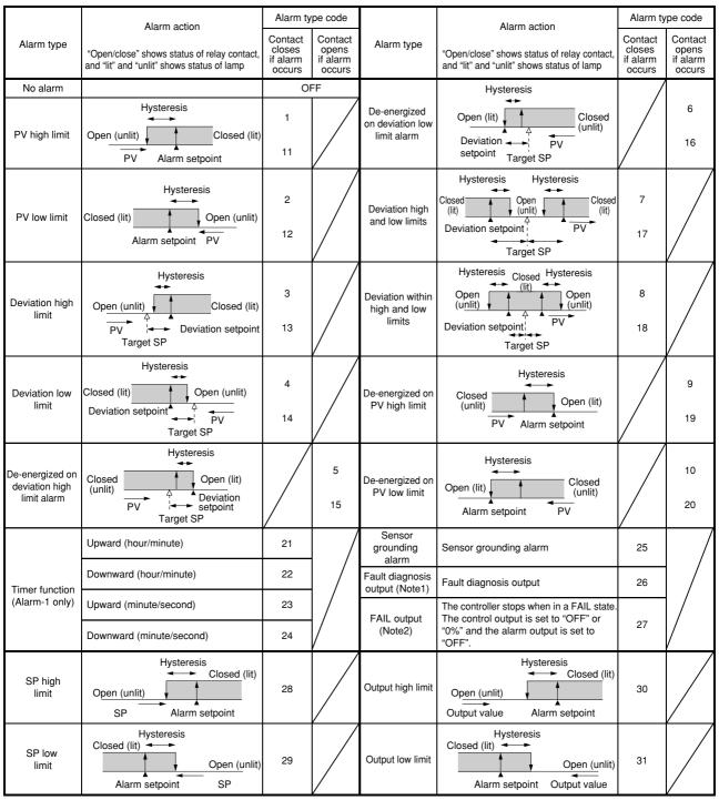
Note 1:The fault diagnosis output turns on in case of input burnout, A/D converter failure, or reference junction compensation (RJC) failure. For input burnout or A/D converter failure, the control output is set to the setpoint of the Preset Output Value operating parameter (PO).
