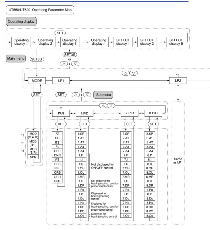
\*1 Parameter MOD (C.A.M.) is displayed when UT mode is "Cascade secondary-loop control", or "Cascade control."
