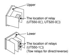
6. Pull out the relay to be replaced. The control output relays are easy to remove and mount, since they are connected via a socket onto the print boards. Insert the new relay in the socket. Use the following relay.
