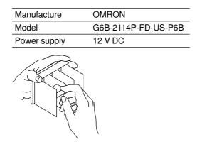
7. Insert the internal unit into the housing. Apply power to the controller and confirm that the initial operating display is shown. If the operating display is not shown properly, turn off the controller and pull out the internal unit. Then, insert it into the housing again.
