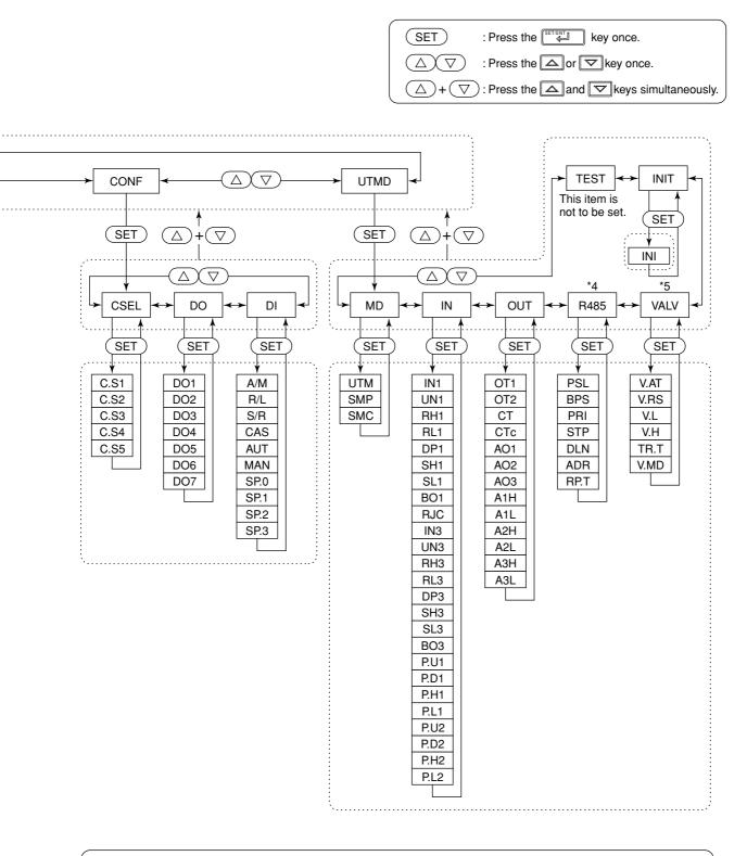
Note: The parameter items shown on the [TEST] submenu of the setup parameter display are to be used by Yokogawa service personnel to check the controller functions. Users cannot set or change these parameters.
