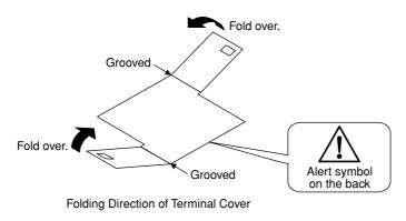
Do not fold the terminal cover the wrong way, doing so not only reduces the cover's strength but may also cause the hinge to crack, thereby disabling attachment.
