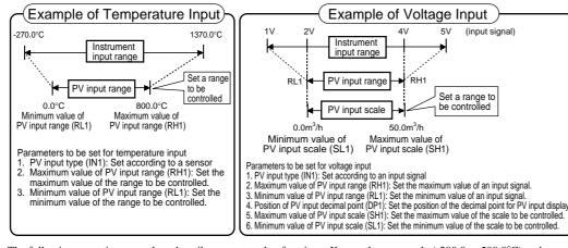
The following operating procedure describes an example of setting a K-type thermocouple (-200.0 to 500.0°C) and a measurement range of 0.0 to 200.0°C.
