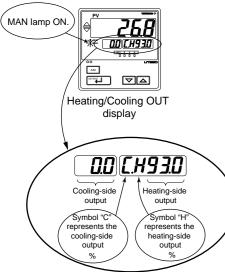
• Controller behavior and control output manipulation when the dead band is positive The following is an example when the DB parameter is set at 12.4%.
