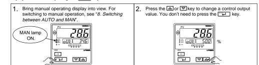
Manipulating the Control Output during Heating/Cooling Control
