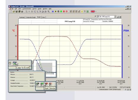
MadgeTech Data Recorder Software displays pressure and temperature data in an easy to use graph.
