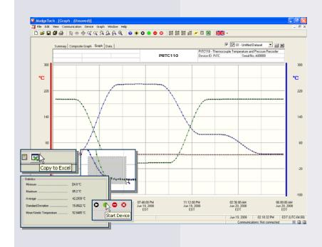
MadgeTech Data Recorder Software displays pressure and temperature data in an easy to use graph.
