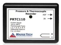
The PRTC110 features a real-time clock module that extends the battery life up to 5 years and allows for high speed downloads. This device will measure and record up to 10,922 measurements per channel. The storage medium is non-volatile solid state memory, providing maximum data security even if the battery becomes discharged. The PRTC110 can be started and stopped directly from your computer and its small size allows it to fit almost anywhere.
