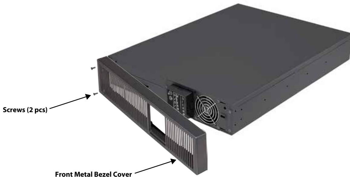
Figure 5: Remove the front metal bezel cover
