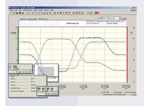
**MadgeTech Data Recorder Software** reports pressure, humidity and temperature data in an easy to use graph.
