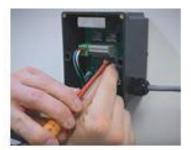
All electrical connections are made inside the junction box. Choose the appropriate cable gland for each connection.
