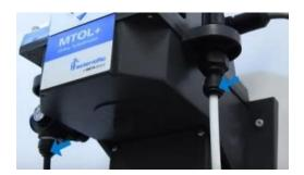
The lower sections of the sensor are equipped with push to connect fittings for use in both the intake and drain. Use ½" OD tubing. Flexible polyethylene or polypropylene tubing is recommended. To lower algae growth opaque tubing is highly encouraged. Make sure the flow through is connected before starting the water flow. We recommended that the flow through be tested for leaks before inserting it into the sensor.
