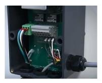
The MTOL+ has outputs for both 4-20mA and Modbus. These are located on grey terminal block on the lower row. The connections are marked on the PCB surface. These spring-loaded terminal blocks are operated by inserting a 3mm (1/8") flat blade screwdriver in the smaller opening directly above the connection. Tilting the screwdriver up will open the connection and allow for wire insertion.
