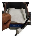
Ensure the provided desiccant is installed in the lower section of the sensor. The sensor can be opened using the four corner thumb screws. The desiccant is simply placed on the lower tray. Ensure the thumb screws are securely tightened to increase desiccant life. DESC will show on the screen when replacement is required.
