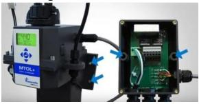
The junction box is located under the sensor portion as shown above. Use appropriate screws and hardware as needed for mounting the instrument to the chosen surface.
