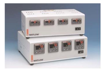
The quad series offers four zones of control in one compact package. Watlow SERIES 935, 93, SD or 96 controls can be utilized for each zone. Each zone utilizes a solid state relay for longer heater life and a lower cost than other power switching devices. The heater output connector can be ordered as either an Amp Mate-'n'-Lok® or a twist and lock connector.
