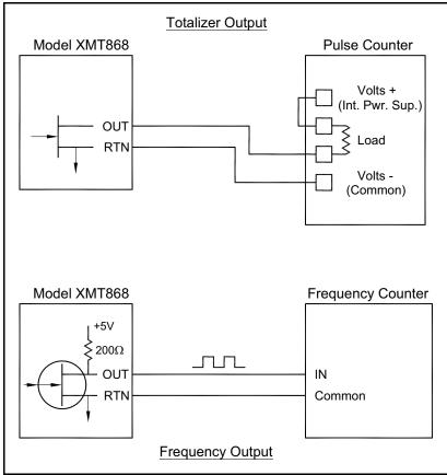
Figure 6: Totalizer and Frequency Output Wiring
