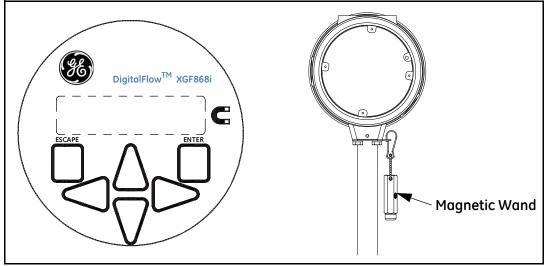
Figure 13: XMT868i Magnetic Keypad and Wand
