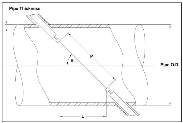
Figure 22: 180° Transducer Installations - Top View
