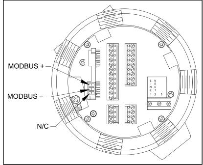
Figure 7: The RS485 MODBUS Terminal Block Connector
