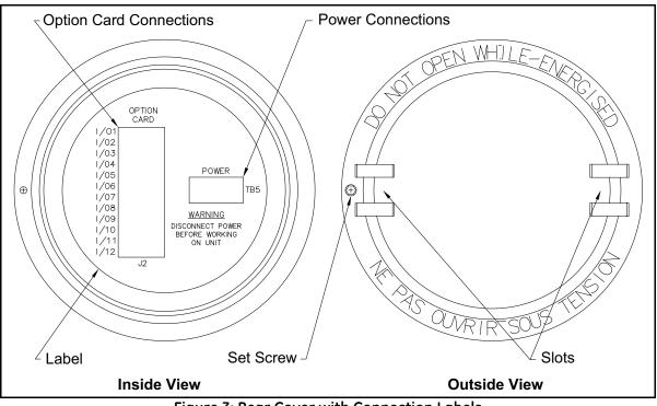
Figure 3: Rear Cover with Connection Labels
