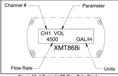
Figure 16: A Typical LCD Flow Rate Display
