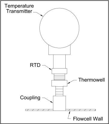
Figure 2: Typical Temperature Transmitter Mounting
