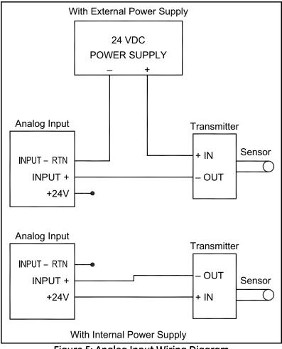
Figure 5: Analog Input Wiring Diagram
