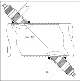
Figure 23: Determining the Pipe Coupling Length
