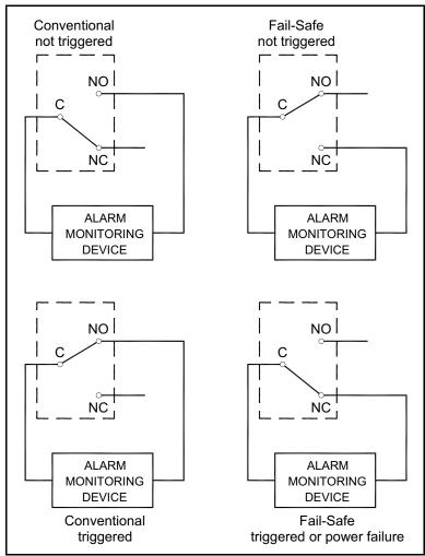
Figure 4: Conventional and Fail-Safe Operation
