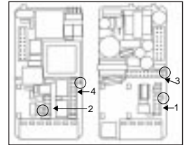
Figure 3 — Main boards and numbered output slots
