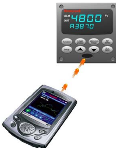
Figure 1-3 Depiction of infrared communications
