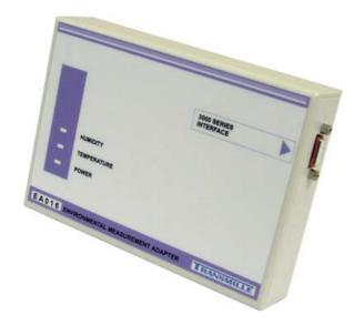
The EA016 provides an easy to use solution for the monitoring of laboratory equipment. It incorporates a robust capacitive humidity sensor with a characterised and linear output and a precision integrated circuit temperature sensor with an output voltage linearly proportional to the Celsius temperature.
