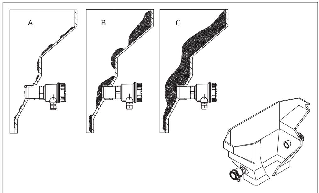
3 Example build-up detection in an electrostatic filter
