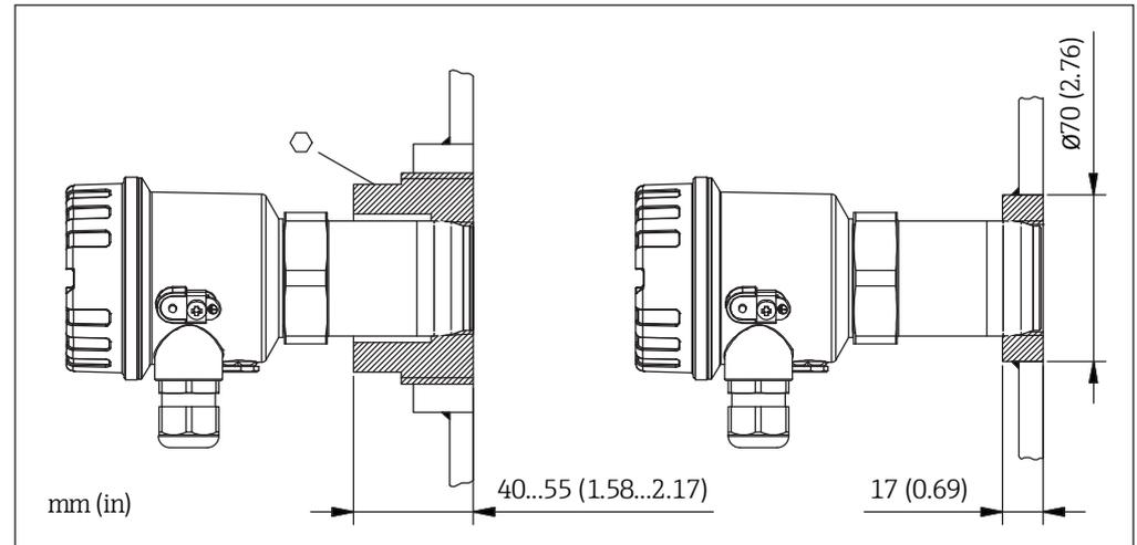
32 Dimensions of weld-in or screw-in adapter FAR52
