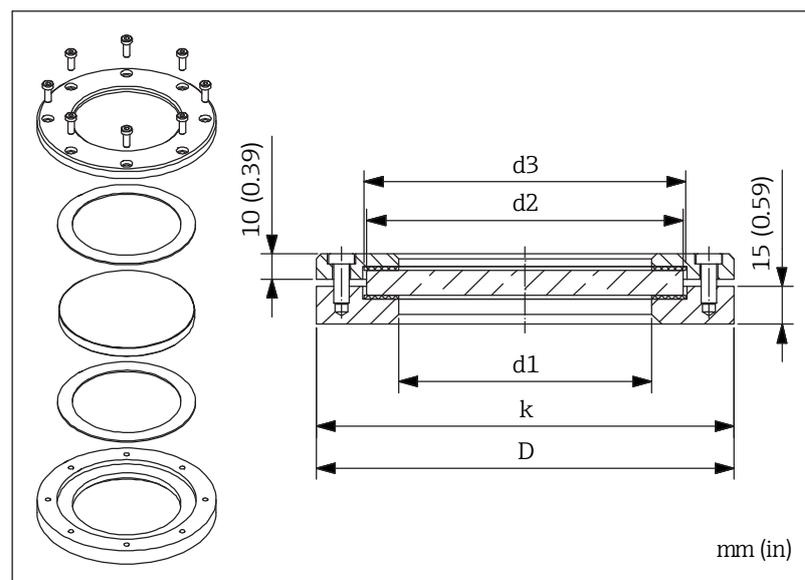
35 Dimensions of sight glass fitting for welding on/in for unpressurized processes
