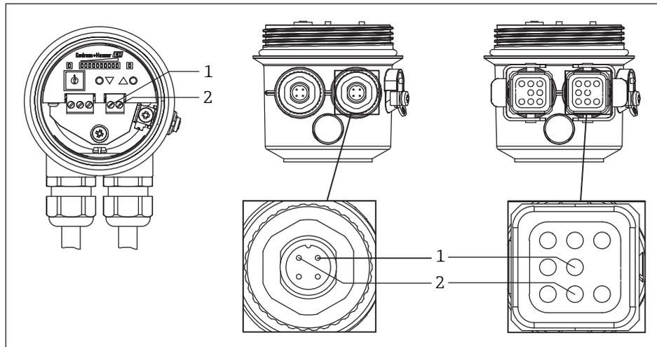
5 Power supply: Terminal and connector assignment (connector 1)
