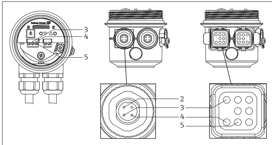
■ 4 Output: Terminal and connector assignment (connector 2)
