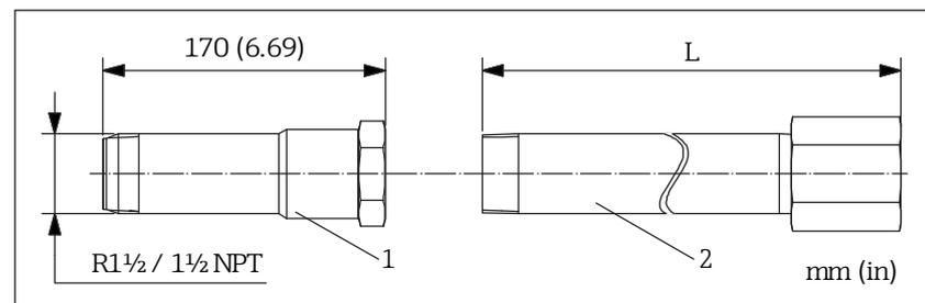
42 Dimensions of high temperature adapter and extensions
