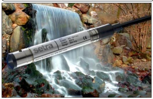
etra System's Model 595 digitally compensated immersible pressure transducer has been specifically designed to meet the rigors of long term immersibility while providing the ultimate in level sensing technology. The 595 has built in specific gravity compensation so it gives a true level reading even when the media is subject to temperature changes over the ranges -5° to +45°C.
