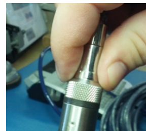
Properly completed—black ring uncompressed
