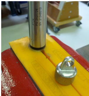
Cableless Sensor—gripping on knurled area
