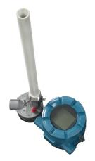
so that both its oxygen probe and the electronics are intrinsically safe without requiring costly design modifications such as flame arrestors. The oxygen probe is constructed of ceramic materials capable of withstanding high process temperatures. Also, the analyzer eliminates the use of the cell heater, using the higher process temperatures to heat the zirconium oxide sensor cell to the temperature required by the Nernst equation principle of operation.
