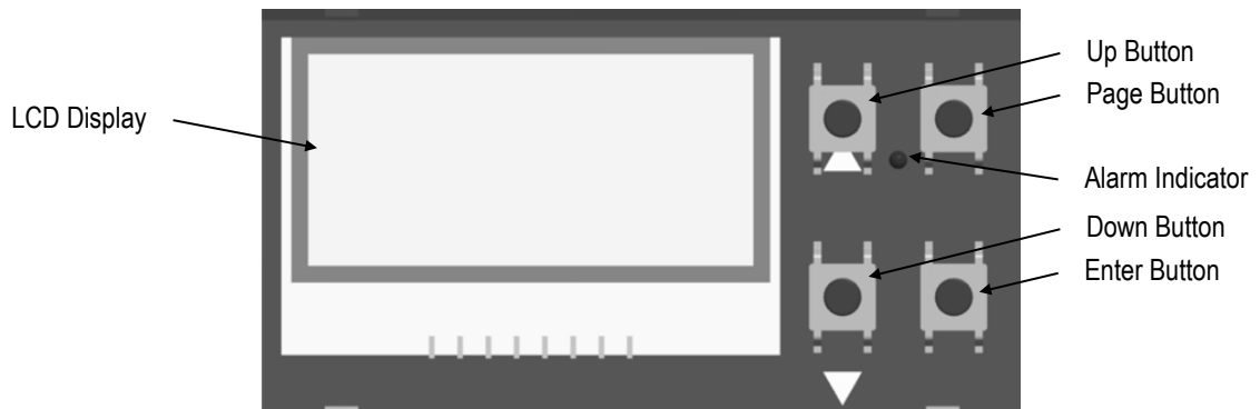
Figure 33: Control Panel for the Comm Box (DIN)
