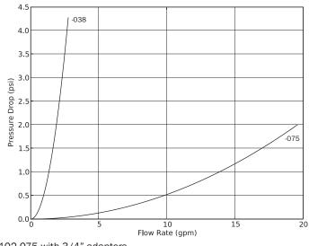
PE102-075 with 3/4" adapters. PE102-038 with 3/8" adapters. Actual curve dependant on pipe size/fittings
