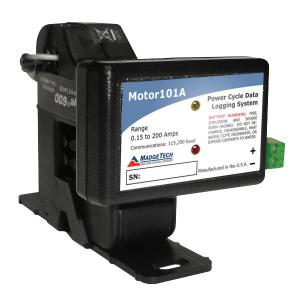
and provides a voltage for the Motor101A to measure. The device can hold up to 406,323 state changes, but memory will only be used if the status has changed. The device can be programmed to check for status changes 4 times per second up to once every 24 hours.
