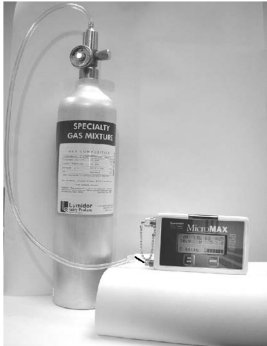
Figure 6 Calibrating the MicroMAX Pro
