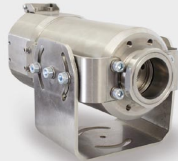
TM-J-CTL Cooling jacket (length 228mm, ø89mm) with adjustable mounting bracket TM-JAB-CTL; up to 200°C ambient temperature
