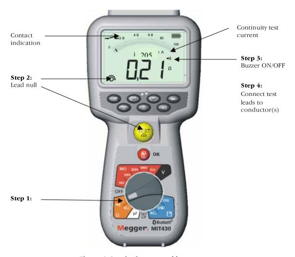
Figure 9 Continuity test and buzzer
