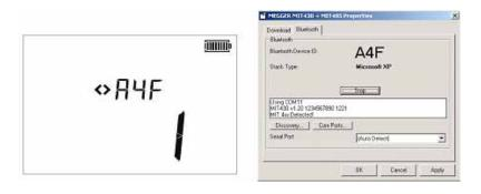
5. With the required address displayed (the three-digit code should match the one displayed on the properties screen) pair the module by pressing the test button until the < > symbols on the auxiliary display alternate.
