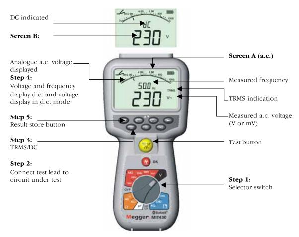
Figure 5 Voltage and frequency measurement
