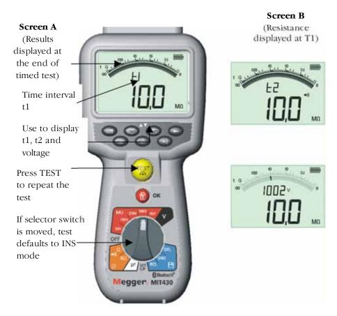
Figure 8 Insulation test - timed mode
