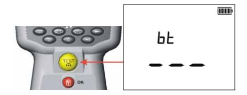
3. Now press and hold the test button until you see the "<" and ">" symbols oscillating. Release the test button. The MIT430 /485 will search for "Bluetooth" computers. At the end of this search, the total number of "Bluetooth" devices will be shown on the main display. The partial address of the last detected device will be shown on the auxiliary display.
