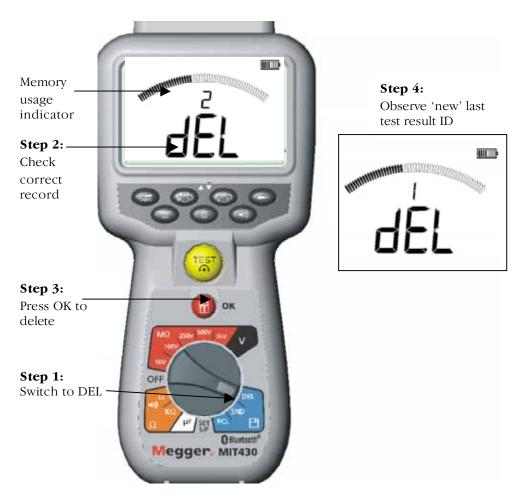
Figure 16 Deleting a single test result
