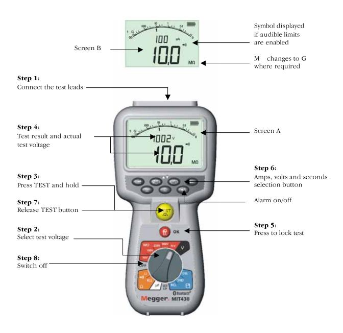
Figure 6 Standard mode insulation test
