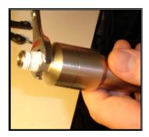
Step 5: Gently slide the PrTrans1000 circuit board from the metal case.
