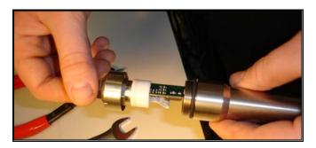
Step 6: Set PrTrans1000 down and make note the orientation of the battery's positive (+) terminal. ( "+" indication is also on the circuit board)
