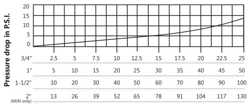
Rate of flow in gallons per minute (GPM)
