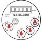
The **3/4" meter** has a fourth dial, as shown above. The x0.01 dial is used for 20 P/G and 10 P/G rates. Note: The 3/4" meter has a 5 digit totalizer.
