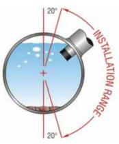
**INSTALL MAGPROBE** BETWEEN 1 0'CLOCK AND 5 0'CLOCK ON THE PIPE
