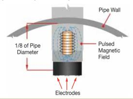
The MFX is the perfect alternative to clamp-on and inline style flow meters where pipe construction and site accessibility may present an installation problem. Dynasonics' "hot-tap" design makes installation of the MagProbe sensor possible without having to plumb in or drain a line.
